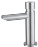
EX316 Self-Closing Push Tap with 1/2" Connection Flow Time 15 seconds (+/- 5 sec) Min. Operating Pressure 2.0 bar MP Brushed Stainless Steel AQE-EX3-304-BS
